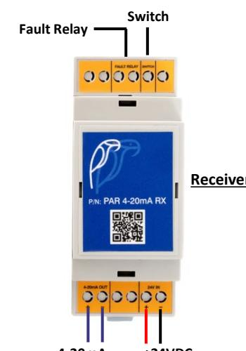
**i** The **Fault relay** is Normally Closed (NC). Change of status occurs when no transmitter signal is received within 2.5 times the transmit interval
